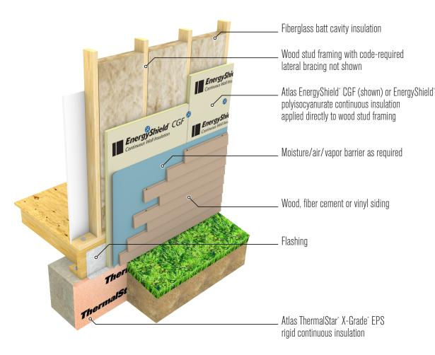
**Note:** Approved lateral bracing methods such as 1"×4" wood let-in-bracing, metal strap cross bracing, inset shear panels and structural sheathing at corners and at regular intervals must be used when polyiso foam is applied directly to wood stud framing. Consult architect, engineer, local code and code official for most appropriate solution.
